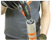
TreeStuff.com suggests a Weaver Premium 12oz. weight. Weights with a thinner shape may not work as desired - a proper seal is important to acheive maximum height and velocity.
