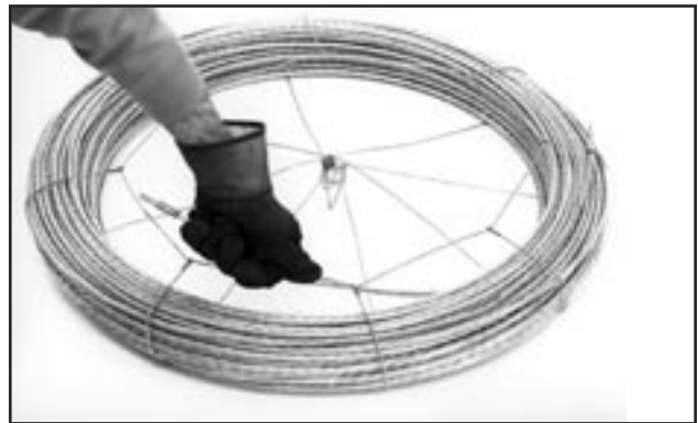
Figure 8 - Secure coil for transport by placing loose end back in dispenser
