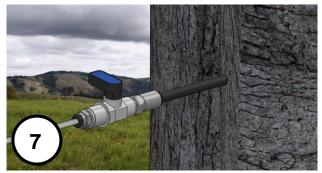
7. <u>Turn OFF</u> valve after tubing has emptied of product. Then wait 10-15 seconds before removing STINGER needle from drill hole.
