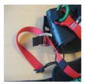
7. Ensure that the two adjuster buckle parts are sitting correctly. Pass the webbing through the slot closest to the waist belt.
