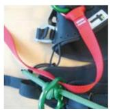
5. Thread the end of the webbing through the upper slot of the front hardware. Take care to ensure that the webbing passes from the middle of the harness toward the outer side of the harness.
