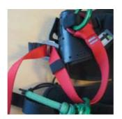
8. Now pass the webbing over the centre rib of the buckle and thread it through the slot closest to the webbing keeper that holds the two buckle parts together.
