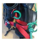
10. Pass the webbing through loop of elastic material again. Before proceeding, ensure that all parts are in the correct place, are not twisted and that the buckles function correctly.
