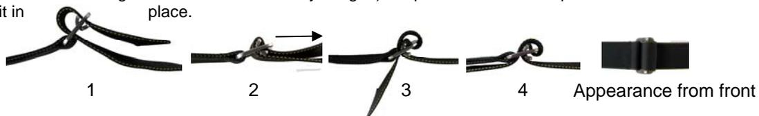
**LEG STRAPS** Bring the leg straps around each leg and fasten the buckles by passing the smaller part through the larger part **from below**. **IMPORTANT: Do not** pass the smaller buckle part through the larger part **from above**. Doing so will allow the webbing to slip and the saddle will fail!
