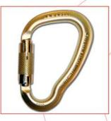
THE NEW BIG DAN HAS A FORGED STEEL BODY WHICH STILL PROVIDES A 50KN/11000LB MBS. IT IS FULLY CE COMPLIANT, NFPA 'G' RATED AND WILL BE AVAILABLE IN AN ANSI 07 FORMAT WITH 3600LB ALL-ROUND GATE STRENGTH. IT WEIGHS A MAXIMUM OF 325G/110Z AND FEATURES A MINIMUM GATE OPENING OF 25MM/1". AS ALWAYS IT IS AVAILABLE IN ALL GATE TYPES FROM SCREWGATE TO 4-WAY QUADLOCK.
