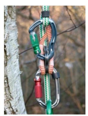
attachment. An Oval karabiner here has the advantage that it can accept wider loads at both ends, so it can be rotated if desired. And the load from the splice is transferred through the rigging plate of the pulley to a central position on the Oval karabiner where the loading pattern is now 1/4-1/2-1/4, which plays to its strengths. Oval karabiners loaded like this often break at well above their rated MBS
